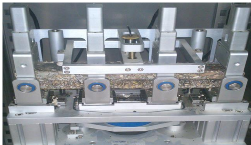
Figure 1. Four-Points Flexural Bending Test Setup
