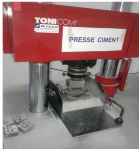
Figure 6. Compression Crushing on a Cement Press Machine
