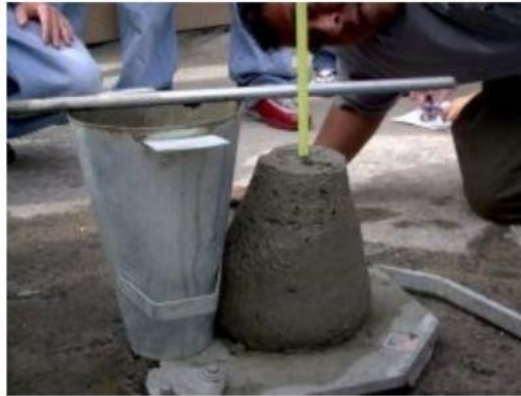
Figure 5. Slump test on mortar
