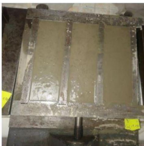
Figure 4. Mortar in a test tube (4 × 4 × 16) cm 3
