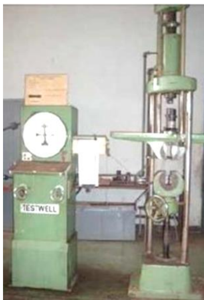
Figure 4. Multifunctional TESTWELL hydraulic press (compaction, maximum strength) at the Ankatso Technical Block
