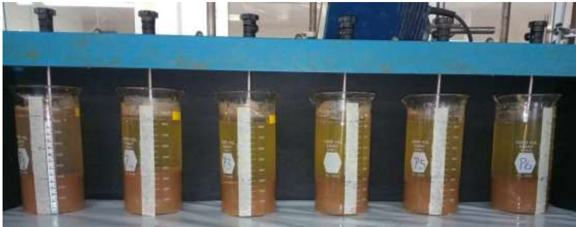
Figure 2. Mechanized jar settling test illustration
