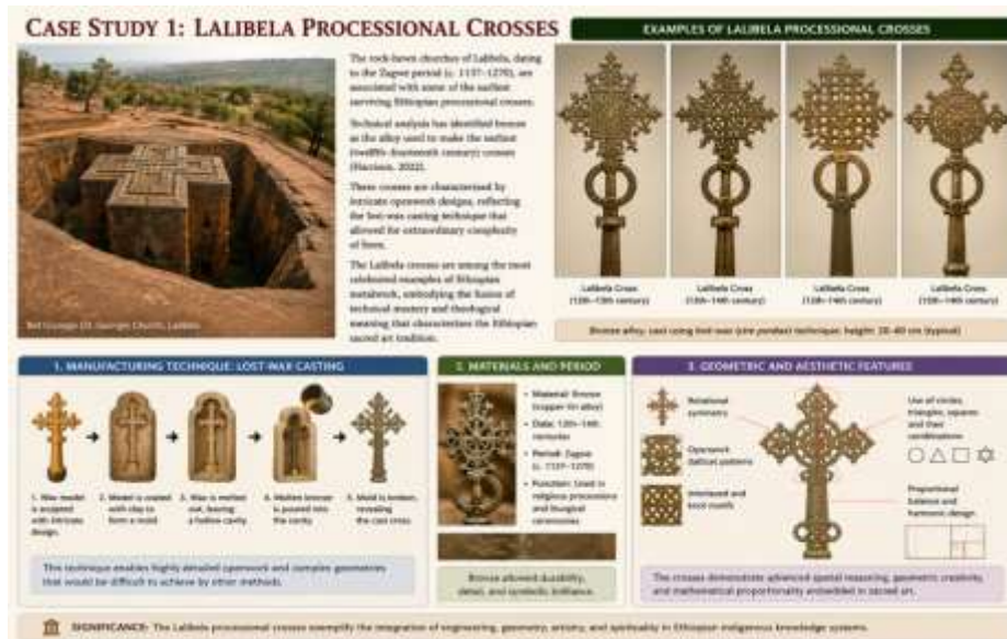
Figure 1. Lalibela processional crosses illustrating advanced lost-wax casting, geometric craftsmanship, bronze metallurgy, and the integration of Ethiopian sacred art and engineering.
